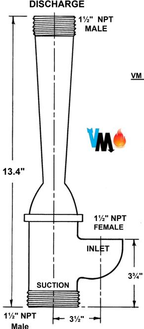
The V.M. # 300-1½"L TYGER Portable Water Eductor will provide a water supply in the absence of functioning fire hydrants. This is accomplished by drafting water from swimming pools, lakes, streams, reservoirs, and other alternate water sources. The Eductor appliance may be utilized where the distance from a water source makes it impractical to draft with hard suction hose. The secondary purpose for the eductor is dewatering basements, boats, tanks etc.
